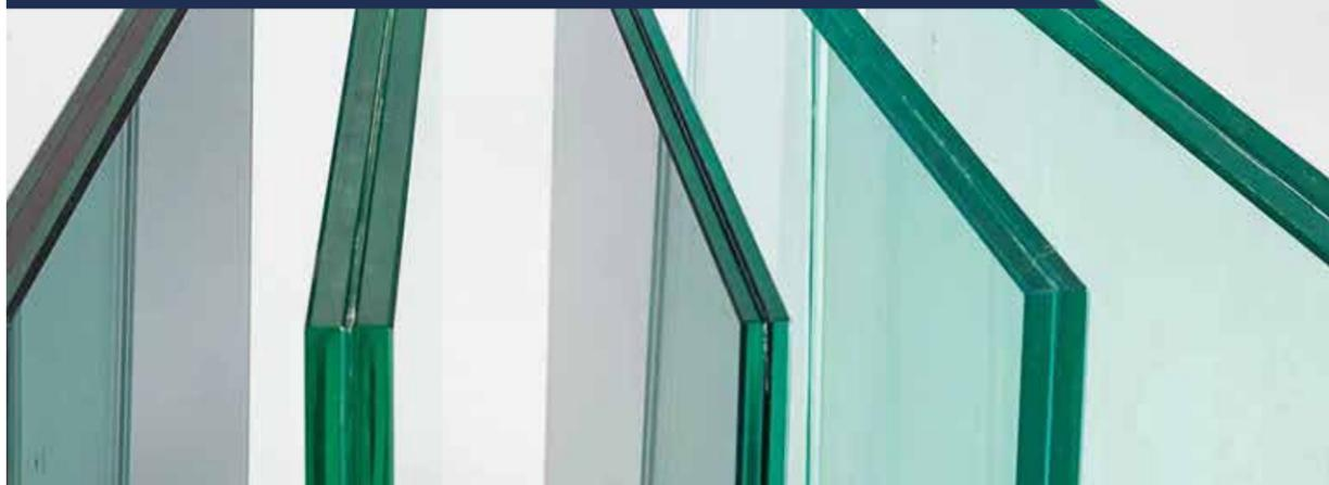
Laminated glass is a glass product composed of two or more pieces of glass. The glass and the intermediate film are permanently bonded together under heat and pressure through the PVB film in the middle of the glass. Compared with tempered glass, which is broken into small particles, laminated glass can still stick together after being broken.
