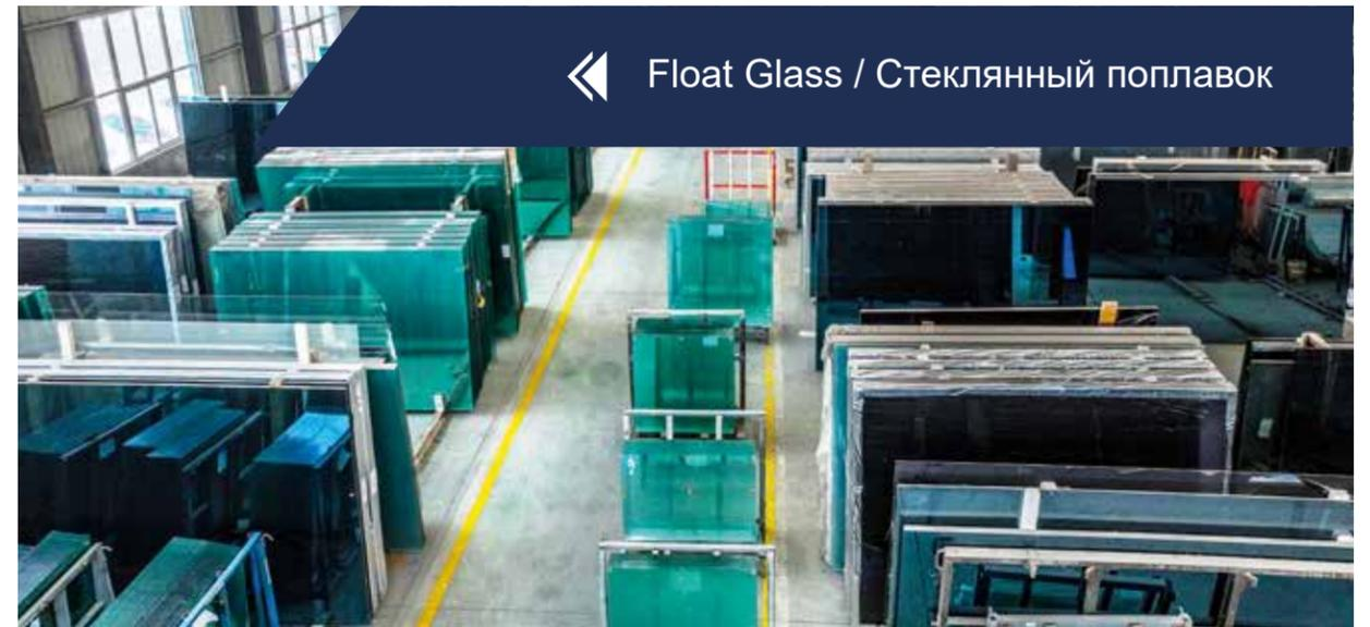
Float glass is made of sea sand, quartz sandstone powder, soda ash, dolomite and other raw materials. It is prepared in a certain proportion and melted at high temperature in the furnace. The molten glass continuously flows from the tank kiln to float on the molten metal surface, and is spread into a fire-polished glass strip with uniform thickness. After cooling and hardening, it separates from the molten metal, and is then annealed and cut to become a transparent colorless flat glass.
